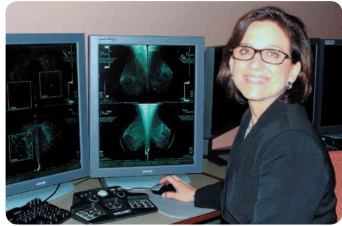
Hologic SecurView diagnostic workstation enables Dr. Bauab to manipulate the digital mammogram electronically to magnify an area, change contrast or alter the brightness of an image.
