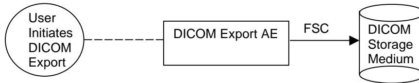
Figure 4.1-1 Application Data Flow Diagram for Media Storage
