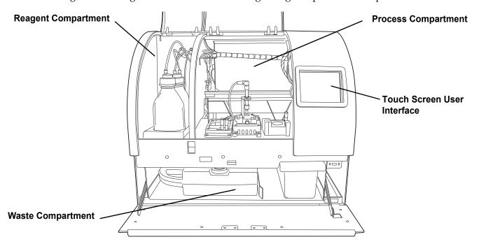
Figure 1-2 Cellient Processor Components
