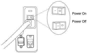
Figure 2-9 Power On/Off Switch
