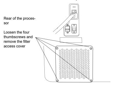
Figure 4-9 Remove the Filter Access Cover
