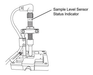
Figure 3-9 Sample Level Sensor (Closed Position)
