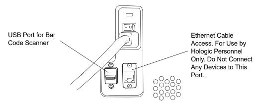
Figure 2-8 USB Port for Bar Code Scanner
