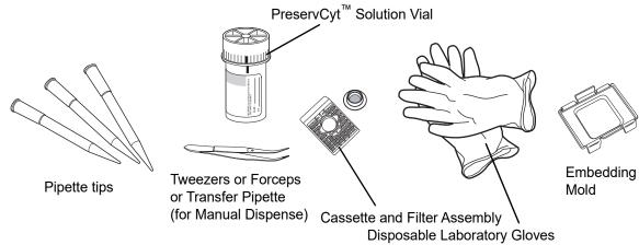
Figure 3-1 Materials Required for Operation
