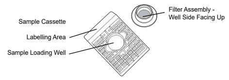
Figure 3-2 Cassette and Filter Assembly - Sample Loading Side
