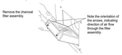
Figure 4-10 Remove the Charcoal Filter
