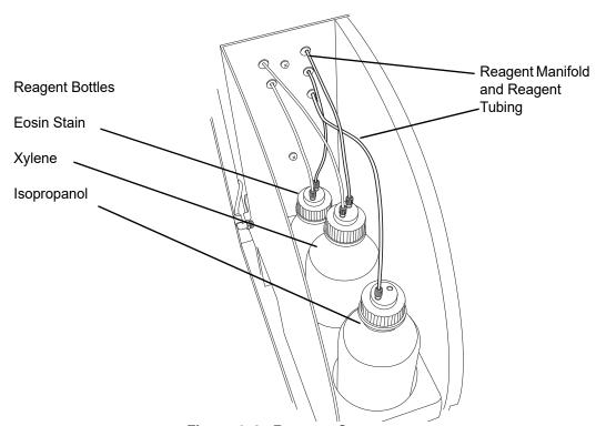
Figure 1-4 Reagent Compartment
