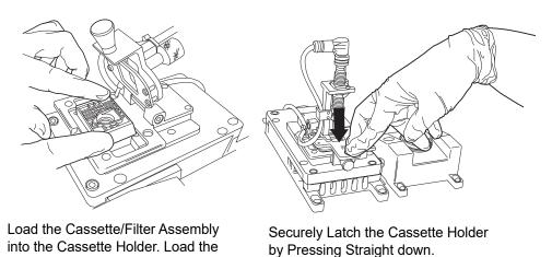
Figure 3-8 Load the Cassette/Filter Assembly into the Cassette Holder
