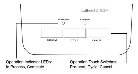
Figure 8-4 Finishing Station Front Panel
