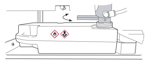
Figure 4-6 Remove/Replace Waste Collection Tank
