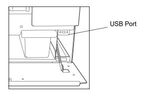
Figure 2-7 USB Port for Downloading Logs
