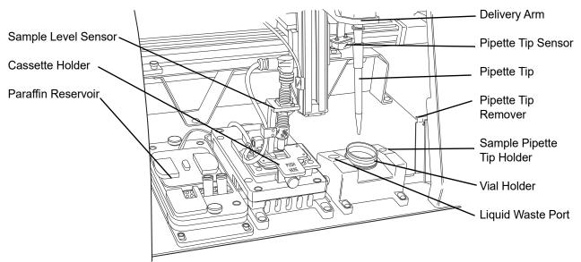
Figure 1-5 Process Compartment Components
