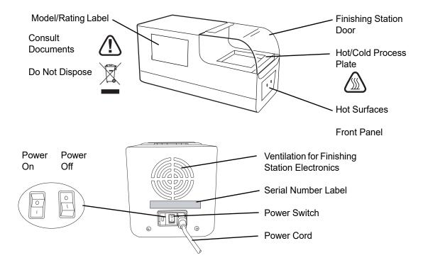
Figure 8-2 Finishing Station Components and Labels
