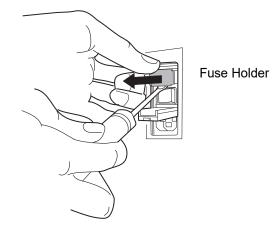
Figure 4-31 Remove the Fuse Holder
