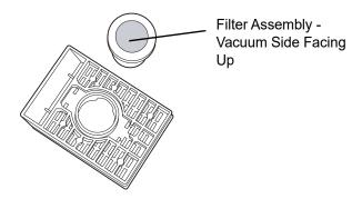
Figure 3-3 Cassette and Filter Assembly - Vacuum Side
