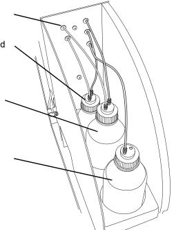
Figure 2-5 Reagent Bottles and Manifold Connectors
