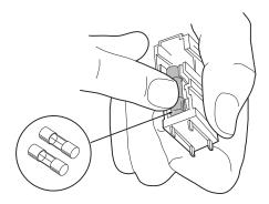
Figure 4-32 Install New Fuses
