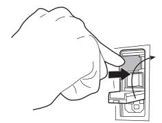
Figure 4-33 Install the Fuse Holder
