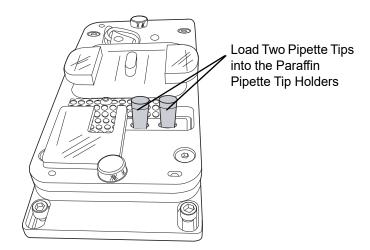
Figure 3-10 Load Paraffin Pipette Tips at Paraffin Reservoir
