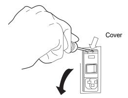
Figure 4-30 Remove Fuse Access Cover
