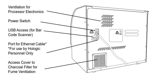
Figure 1-3 Cellient Processor - Rear
