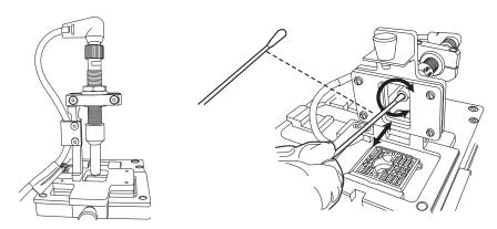
Figure 4-8 Clean the Sample Level Sensor
