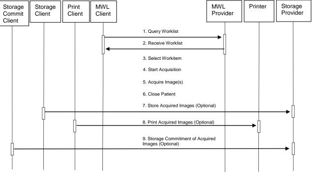
Figure 3.1-1: Image Acquisition Sequence Diagram
