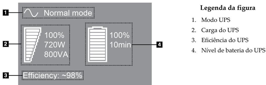
Figura 111: Monitor de LCD do UPS
