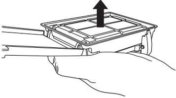
A line drawing showing a hand holding the slide box, with an upward-pointing arrow indicating it is being lifted away from the cassette.                     |
