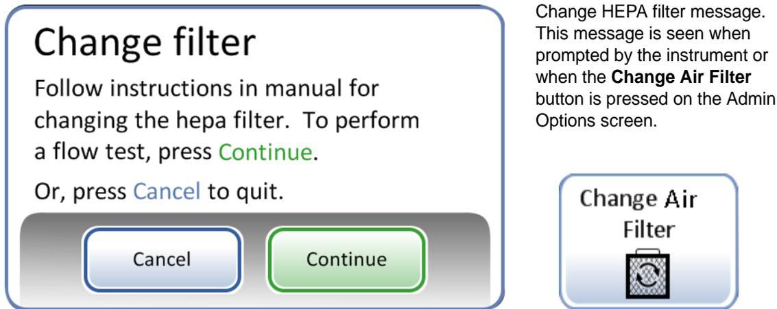
Change HEPA filter message. This message is seen when prompted by the instrument or when the **Change Air Filter** button is pressed on the Admin Options screen.
