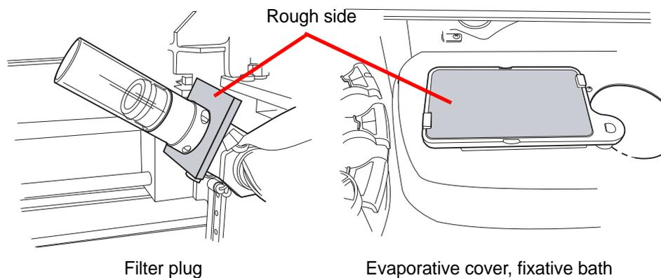
**Figure 8-17 Absorbent Pads**
