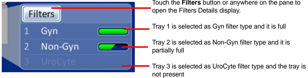
Figure 6-13 Filters Pane on the Main Screen
