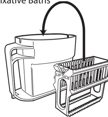
Fixative baths - orient the staining rack so that the embossed words "UP SIDE" face the bath handle. Press the staining rack all the way down until it can be felt to snap into place. The rack must be fully seated.
