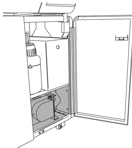
The fume extractor is located at the bottom of the waste cabinet of the AutoLoader.
