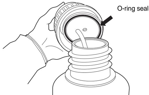
**Figure 8-13** Inspect Waste Bottle O-Ring Seal
