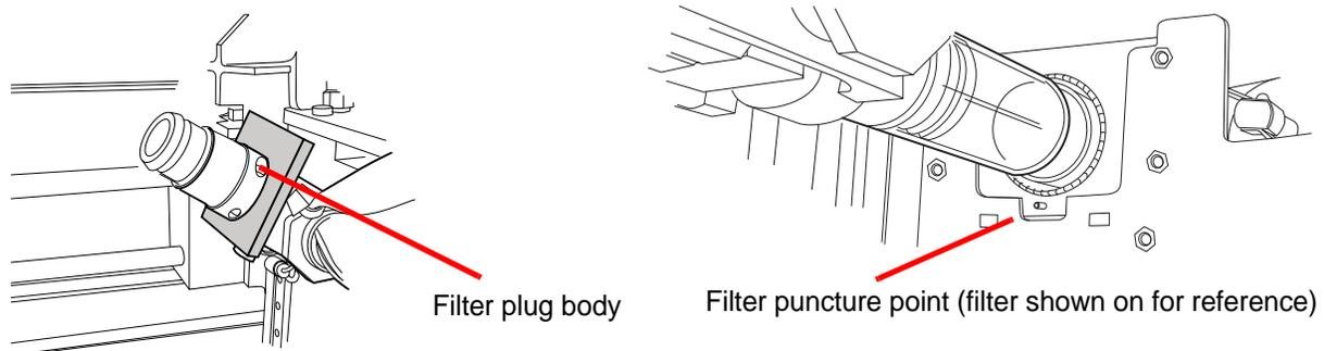
Figure 8-4 Clean Filter Plug and Filter Puncture Area
