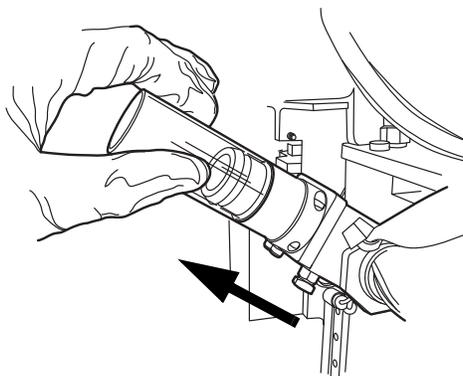
Figure 9-4 Release Filter
