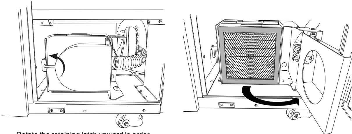
Rotate the retaining latch upward in order to open the door.
