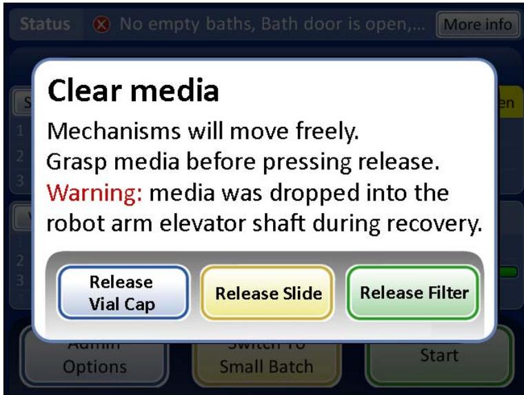
**Release Vial Cap** will open the fingers of the vial gripper to drop the vial cap
