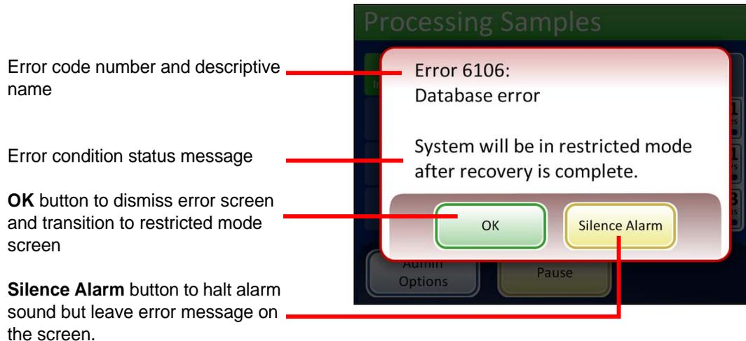
Figure 9-1 System Detected an Error
