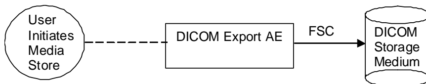
Figure 5.1-1: Application Data Flow Diagram for Media Storage
