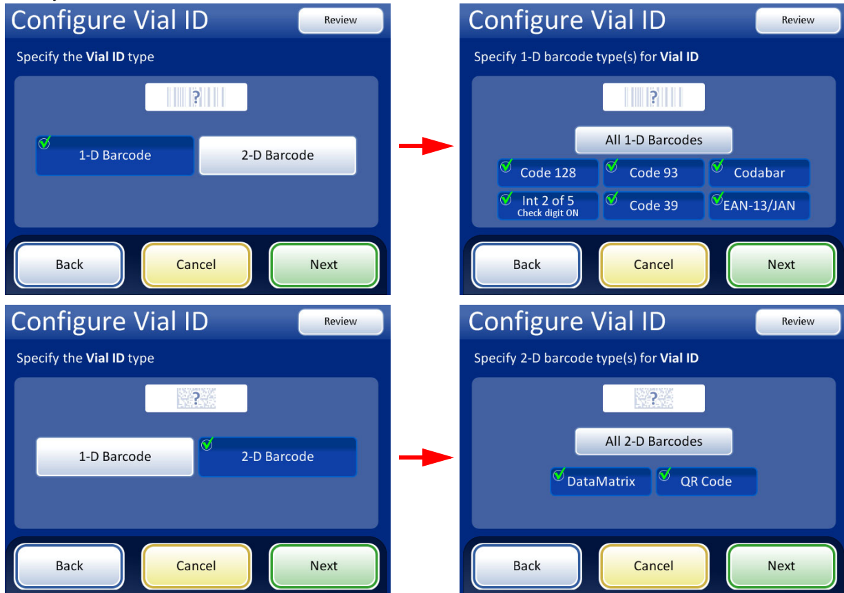
Figure 6-37 Configure Vial ID barcode type(s)
