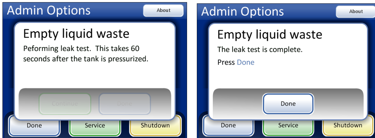
Figure 8-15 Waste System Leak Test
