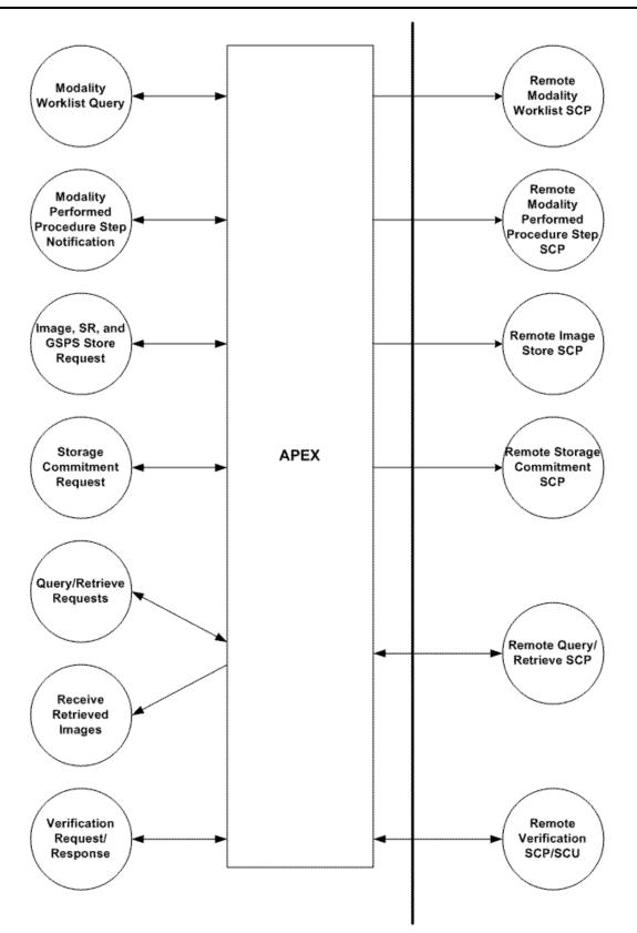
Figure 4.1-1. Application Data Flow Diagram
