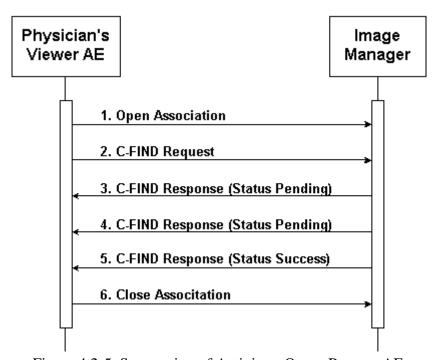
Figure 4.2-5. Sequencing of Activity – Query Remote AE
