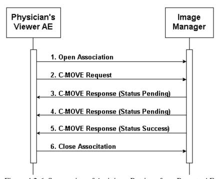
Figure 4.2-6. Sequencing of Activity – Retrieve from Remote AE
