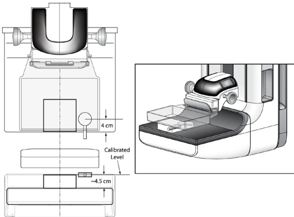
Figure 3: ACR Phantom and Ionization Chamber Setup
