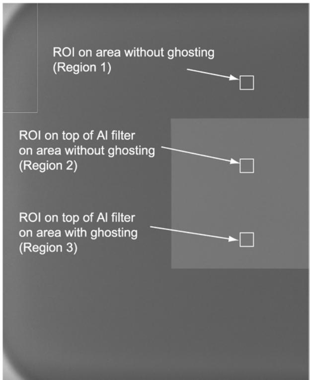
*Figure 7: Preview Screen Showing Set-up for Detector Ghosting Test*
