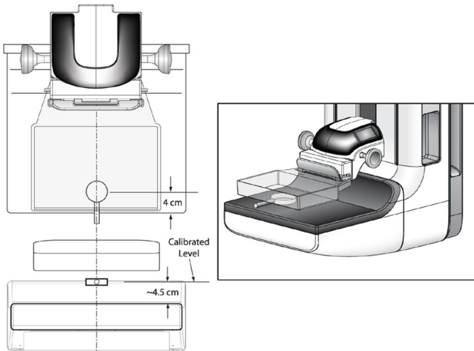
Figure 4: Centered Ionization Chamber
