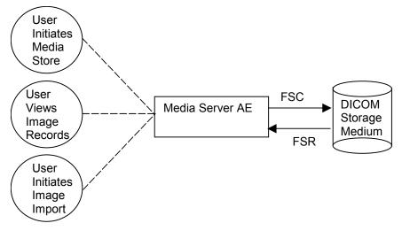
Figure 4.1-1 Application Data Flow Diagram for Media Storage
