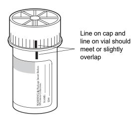
Figure 3-1 Aligning the Vial Cap
