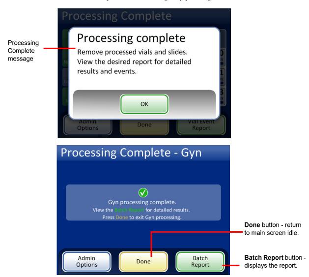
Figure 6-12 Processing Complete Screen
