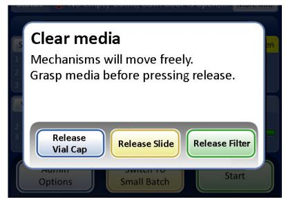
**Release Vial Cap** will open the fingers of the vial gripper to drop the vial cap.
