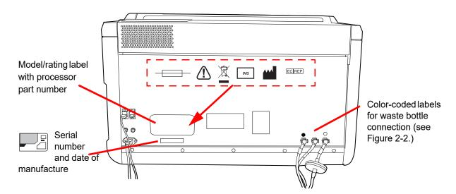
Figure 1-7 Rear of the ThinPrep™ 5000 Processor
