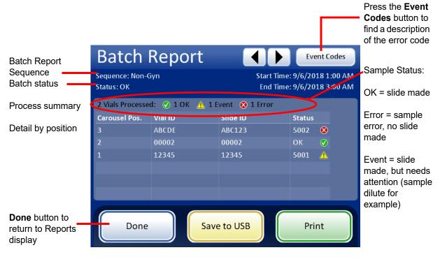
Figure 6-59 A Batch Report Display - Successful Batch
