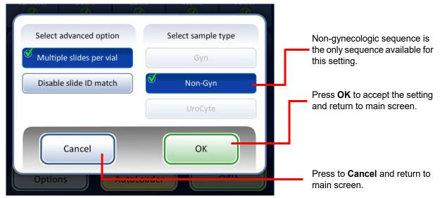
Figure 6-5 Multiple Slides per Vial Screen
