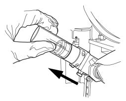
Figure 9-4 Release Filter
