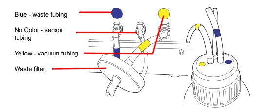
Figure 8-13 Waste Bottle Tubing Connections
