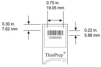
Figure 7-4 Barcode Slide Label Format
