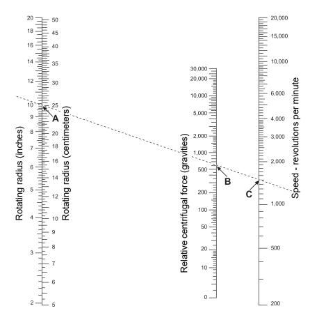
Figure 5-2 Determining the Correct Centrifuge Speed
