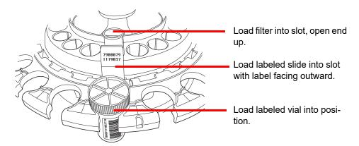
Figure 7-7 Load Carousel with Vials, Slides and Filters
