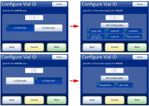
Figure 6-37 Configure Vial ID barcode type(s)
