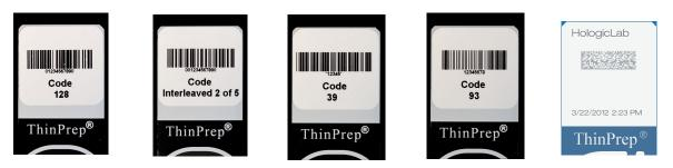
Figure 7-3 Examples of How Barcodes Fit onto a ThinPrep Slide
