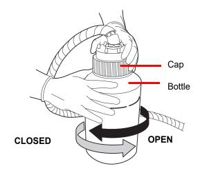
Figure 8-10 Opening/Closing the Waste Bottle
