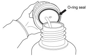
Figure 8-11 Inspect Waste Bottle O-Ring Seal
