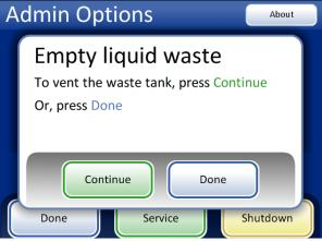
Figure 8-7 Empty Liquid Waste Button and Message
