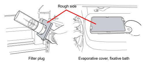
Figure 8-15 Absorbent Pads
