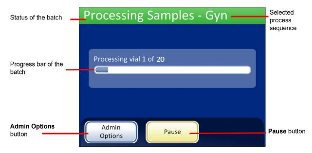
Figure 7-14 Starting the Batch Screen
