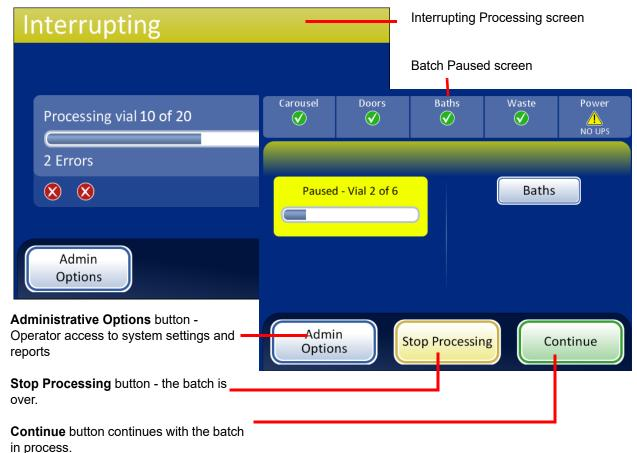
Figure 6-11 Processing Paused Screen
