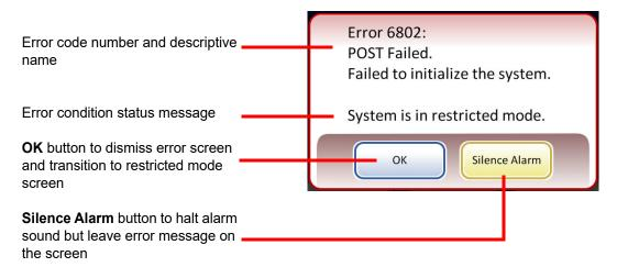
Figure 9-1 System Detected an Error
