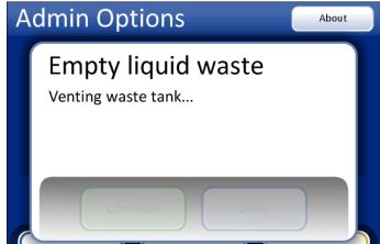
Figure 8-8 Venting the Waste Bottle
