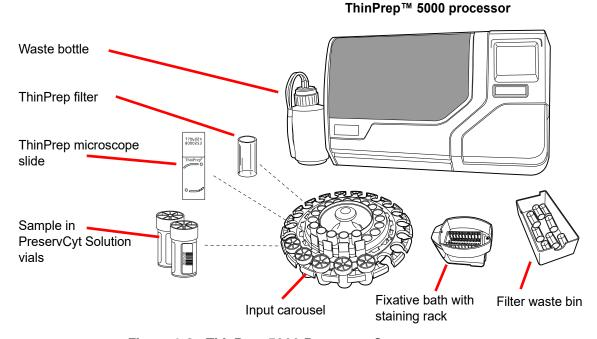
Figure 1-3 ThinPrep 5000 Processor Components
