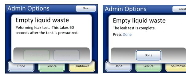
Figure 8-12 Waste System Leak Test
