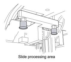
Figure 8-5 Clean Slide Holder Pneumatic Suction Cups
