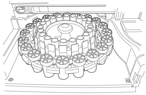
Figure 7-9 Load Carousel into the Processor
