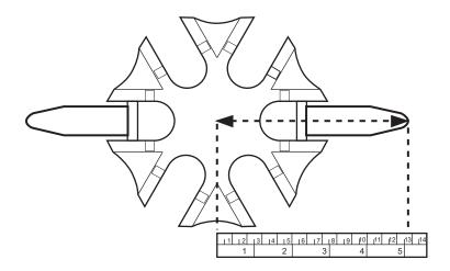
Figure 5-1 Measuring the Centrifuge
