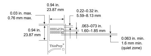
Figure 7-6 Slide OCR Label Formats
