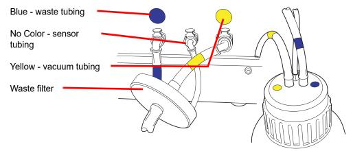
Figure 2-2 Waste Bottle Tubing Connections
