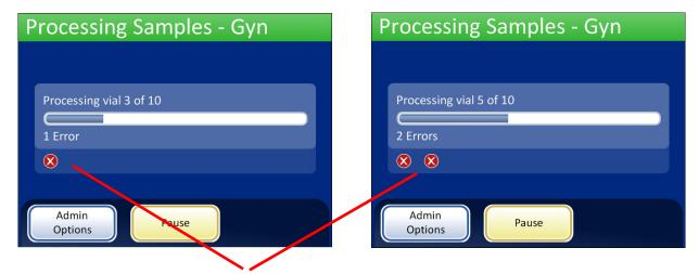
Sample error indicators are displayed on the screen during processing.
