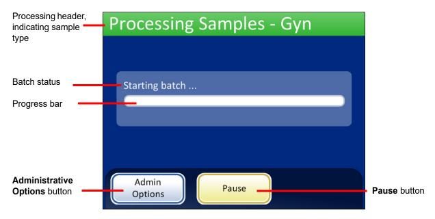
Figure 6-8 Starting Batch Screen
