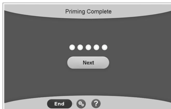
After successfully priming the Fluent Fluid Management System, it is ready to operate during a procedure. System does not need to be zeroed after priming if priming was done inside the under-buttocks drape. If priming was done outside of the under-buttocks drape the fluid deficit needs to be zeroed as a false deficit can ensue.
