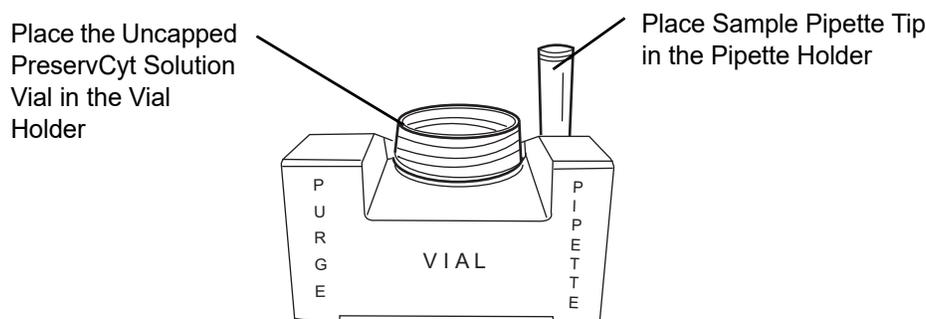
**Figure 3-7 Load Sample Vial and Sample Pipette Tip**
