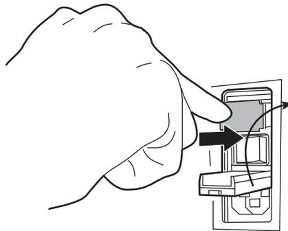
**Figure 4-33 Install the Fuse Holder**
