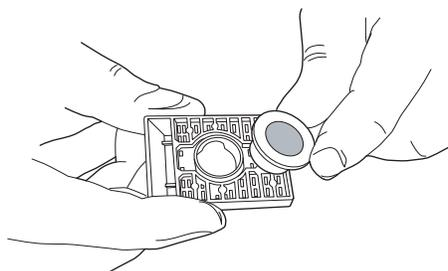
**Figure 3-4 Press Filter Assembly Onto Cassette - Vacuum Side**
