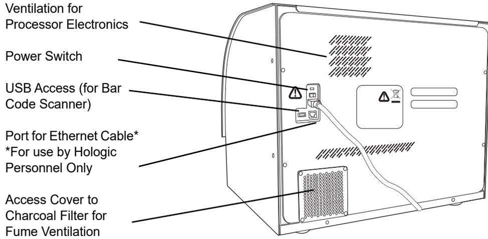
**Figure 1-3 Cellient Processor - Rear**
