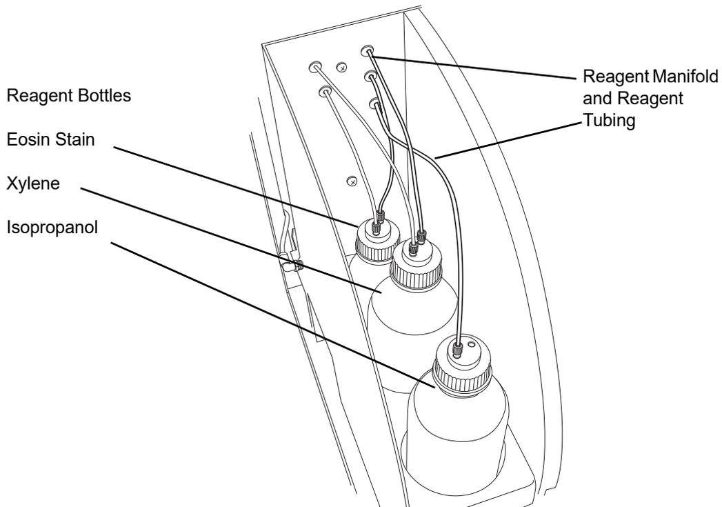
**Figure 1-4 Reagent Compartment**
