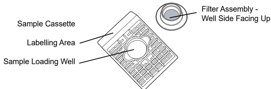
**Figure 3-2 Cassette and Filter Assembly - Sample Loading Side**
