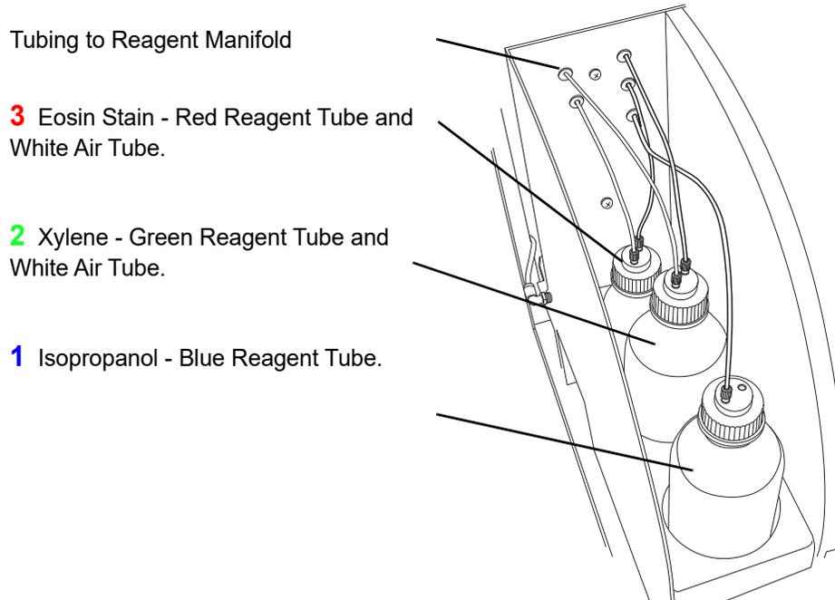
**Figure 2-5 Reagent Bottles and Manifold Connectors**
