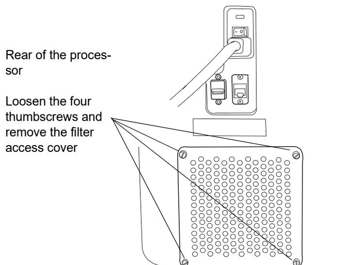
**Figure 4-9 Remove the Filter Access Cover**
