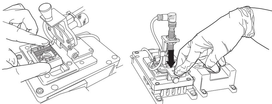
Load the Cassette/Filter Assembly into the Cassette Holder. Load the Assembly with the Filter Side Down.
