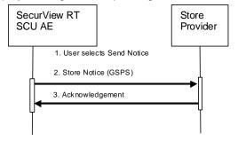
Figure 4.1-3: Send Notice Sequence Diagram
