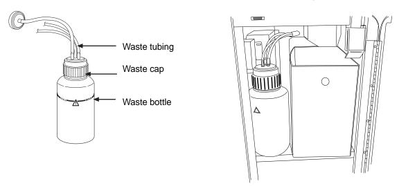
Figure 8-8 Waste Bottle and Waste Bottle Location
