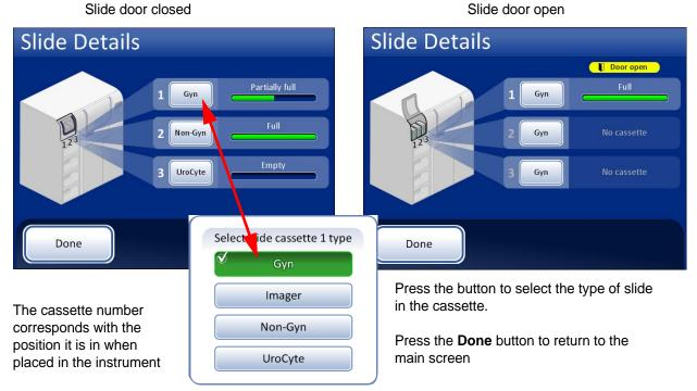
Figure 6-5 Slide Details Display
