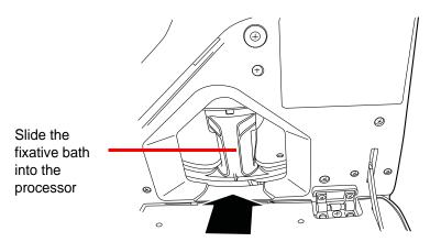
Figure 7-10 Load Fixative Bath into the Processor
