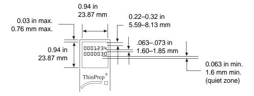
Figure 7-22 Slide OCR Label Formats
