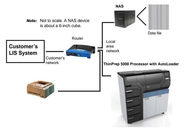
Figure 2-2 Local Network Interconnection Schematic (Example)
