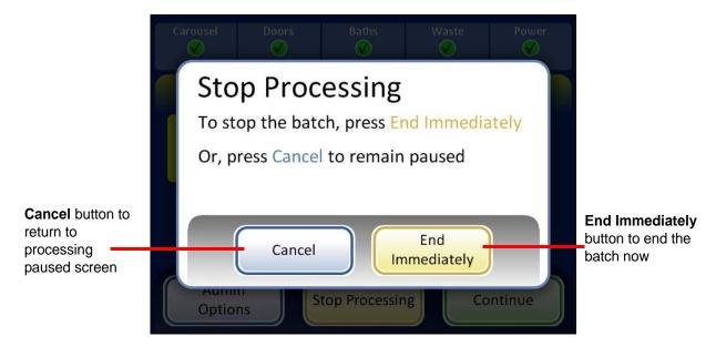
Figure 7-33 Stop Processing Screen
