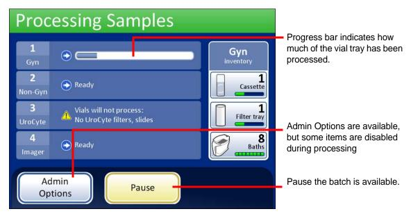
Figure 7-14 Processing Samples Screen
