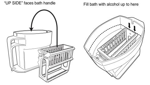
Figure 7-9 Fixative Bath and Staining Rack
