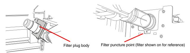
Figure 8-4 Clean Filter Plug and Filter Puncture Area
