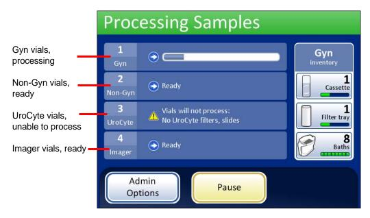
Figure 6-17 Processing Samples Screen
