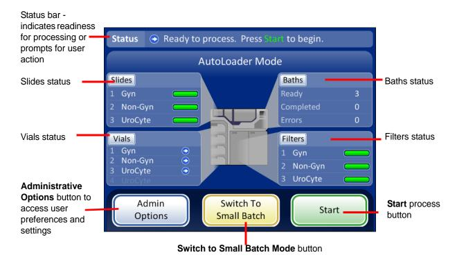
Figure 6-1 Main Screen, Status Ready to Process
