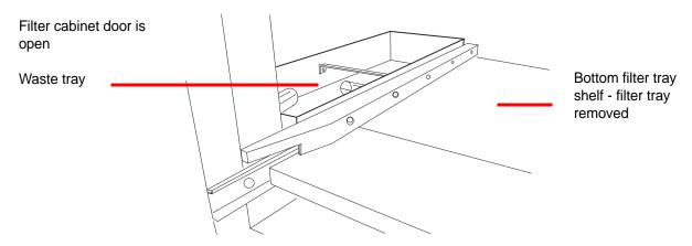
Figure 9-8 Robotic Arm Elevator Shaft Waste Tray
