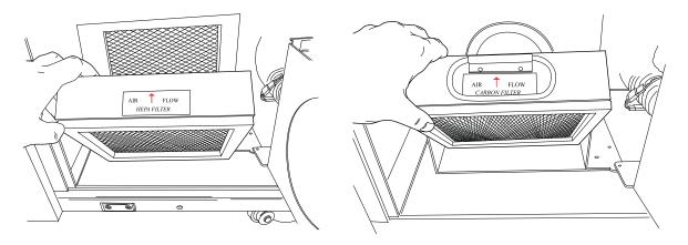
Figure 8-21 Remove the HEPA and Carbon Filters
