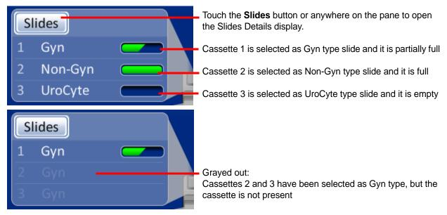
Figure 6-4 Slides Pane on Main Screen
