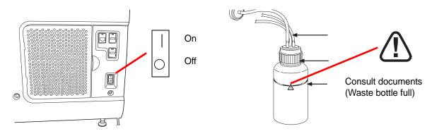
Figure 1-8 Right Side of Processor and Waste Bottle
