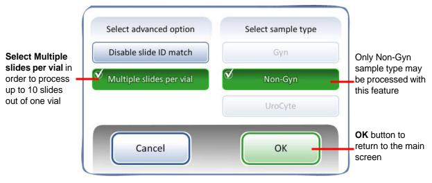
Figure 7-27 Multiple Slides per Vial
