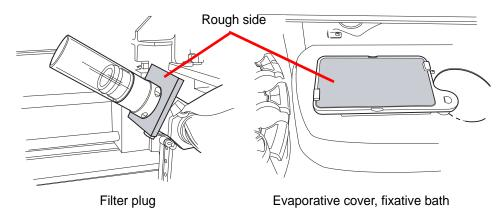
Figure 8-17 Absorbent Pads
