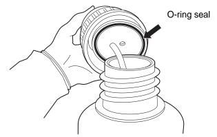
Figure 8-13 Inspect Waste Bottle O-Ring Seal
