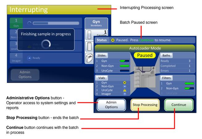
Figure 6-22 Processing Paused Screen
