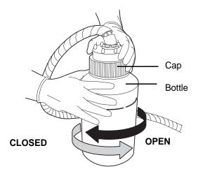
Figure 8-12 Opening/Closing the Waste Bottle
