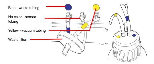
Figure 8-15 Waste Bottle Tubing Connections
