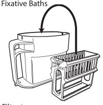
Fixative baths - orient the staining rack so that the emobssed words "UP SIDE" face the bath handle. Press the staining rack all the way down until it can be felt to snap into place. The rack must be fully seated.
