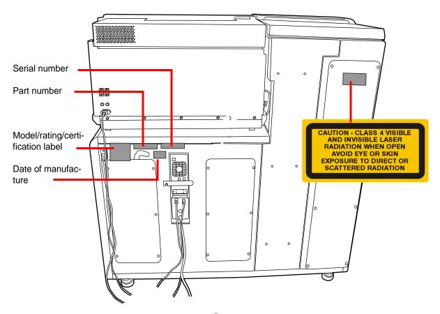
Figure 1-7 Rear of the ThinPrep® 5000 Processor with AutoLoader
