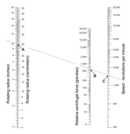
Figure 5-2 Determining the Correct Centrifuge Speed
