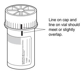
Figure 3-1 Aligning the vial cap
