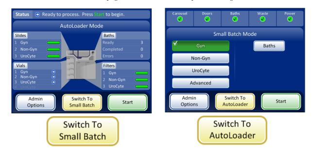
Figure 6-24 Switch Mode Buttons
