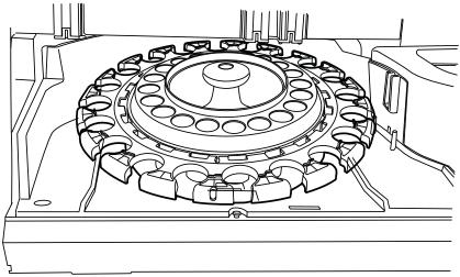
Figure 7-11 Load Carousel into the Processor
