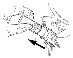
Figure 9-4 Release Filter
