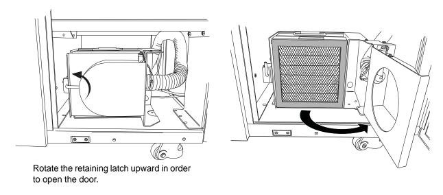
Figure 8-20 Open the Fume Extractor Door
