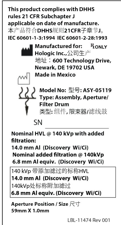
Figure 23 Discovery Wi, Ci Radiation Compliance/Aperture Size Label
