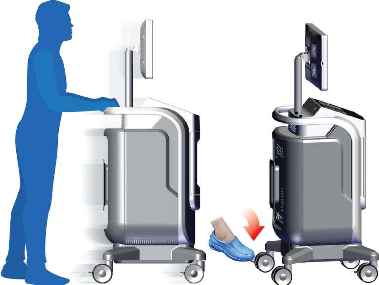
The diagram illustrates the first step of the sequence. On the left, a blue silhouette of a person is shown standing next to the console, which is on a swivel castor. The person's hands are on the console, and a red arrow points to the right, indicating movement. On the right, the console is shown in its final position, with a red arrow pointing down to the castor, indicating that it should be locked. |
