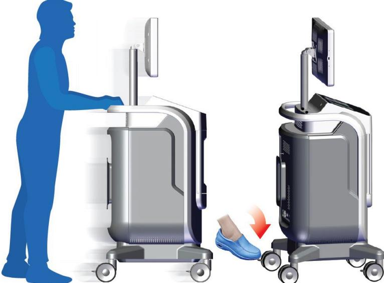
The diagram illustrates the first step of the sequence. On the left, a blue silhouette of a person is shown from the side, standing next to the Trident HD console. The person's hands are on the console's control panel. On the right, the console is shown in its final position. A red arrow points from the person's foot towards the front casters of the console, indicating the action of locking them. |
