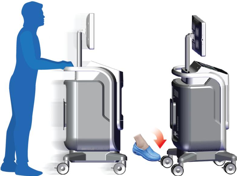
The diagram illustrates the first step of the sequence. On the left, a blue silhouette of a person is shown standing next to the mobile X-ray console. The person's hands are on the console, and a red arrow points to the right, indicating movement. On the right, the console is shown in its final position. A red arrow points down to the front casters, indicating they are to be locked.   |
