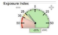
The implementation of the algorithm for the EI Gauge may present an incorrect indication when used with any DBT image derived from 1X1 binning.
