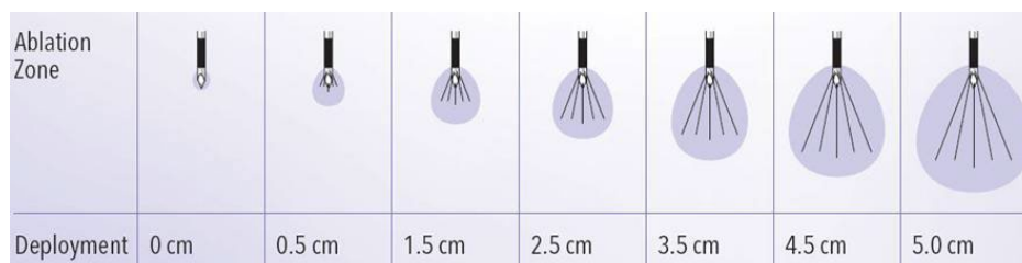
Figure 12-1 Representative Ablation Shape per Deployment
