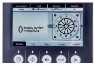
Once the "Test" cycle is complete, you can follow the prompts to test "Arm" and "Fire" or you can proceed to "Standby".
