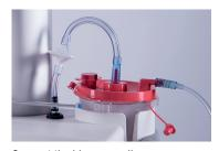
Connect the biopsy needle vacuum tubing to the "PATIENT" port of the canister lid.
