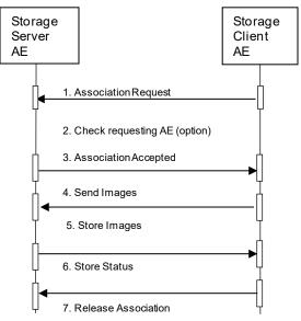
Figure 3.1-3: Storage Sequence Diagram
