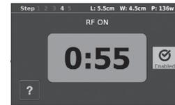
**NOTE: RF power delivery can be stopped at any time by pressing the foot switch.**
