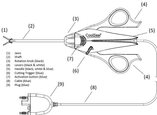
1. Remove instrument from tray by firmly pulling on the handle (5). Do not pull on the instrument's jaws (1), shaft (2), or cable (8).
