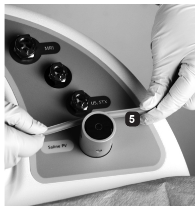
FIGURE 6: SALINE PINCH VALVE CONNECTION
