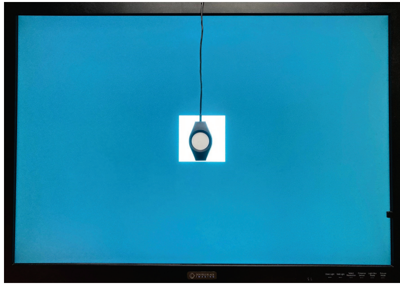
Figure 27: Using an External Photometer During Annual Physicists Testing
