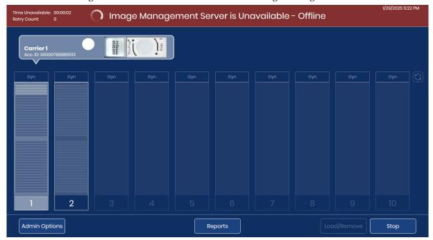
Figure 1-6-1 No connection between Image Management Server and Digital Imager
