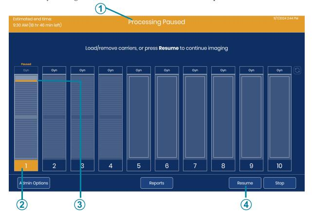
Figure 1-4-18 Slide processing paused
