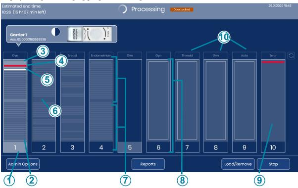
Figure 1-3-4 Screen display indicates slide carrier position
