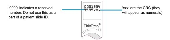
Figure 1-4-5 Accession ID in OCR format
