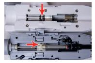
Ensure biopsy needle and driver are in the ready position before assembly. To reset driver (if needed), disconnect and plug into the console. To reset biopsy needle, manually slide white gear forward until it clicks into place.
