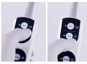
OPTIONAL: To "Arm" press and hold Arm button. To "Fire" press and hold Fire button. System will default to "Standby" when complete.
