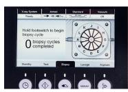
Select "Biopsy" mode and "Arm" device. Confirm appropriate aperture (12mm or 20mm) and needle position is displayed on both screens. The device will only "Arm" and "Fire" in "Biopsy" mode.
