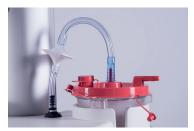
Securely connect the blue fitting of the Vacuum Line Assembly to the "VACUUM" port.
