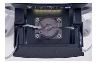
Open the drawer and click the tissue filter assembly into place, routing the tubing through the guides. Ensure tissue filter cap is secure. Close the drawer.
