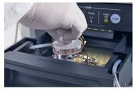
Open drawer. Twist off the tissue filter assembly cover. Place a cap on the tissue filter. Remove filter and place in a formalin jar. Replace the tissue filter assembly cover.
