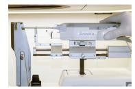
Attach Brevera adapter to imaging guidance system. Slide the biopsy device onto the adapter until it clicks in place. Confirm appropriate settings on the imaging system for the chosen biopsy needle.
