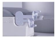
To begin biopsy, place introducer onto needle in the 20mm or 12mm aperture position. System will not function if introducer is not installed.
