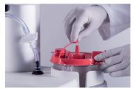
Disconnect the Vacuum Line Assembly from the canister lid and seal all ports.
