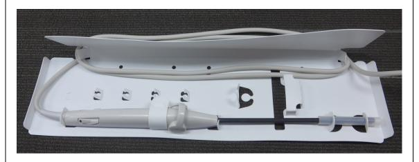
Carefully insert the electrical connector into its constraint on the backer card
