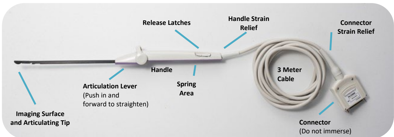
Figure 1-1 Relevant components of the IUUS Probe.
