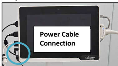
Figure 3-3. Power Cable connection to the SMART Tablet.
