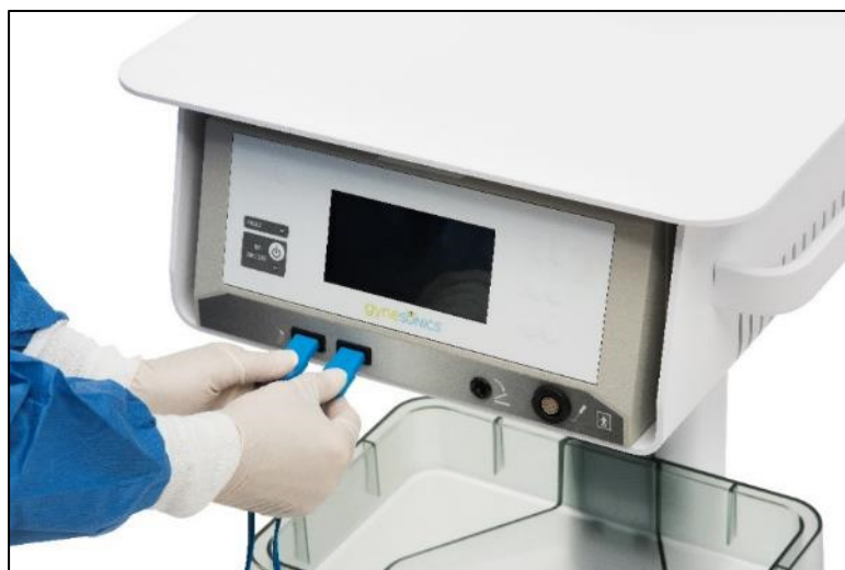
Figure 3-15. Connect both Dispersive Electrode cables to the front of the RF Generator.
