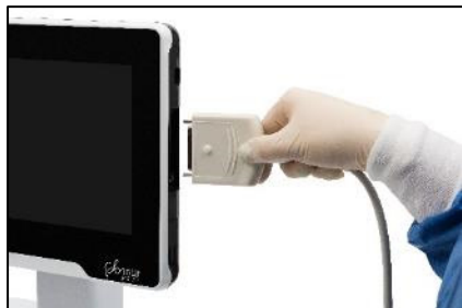
Figure 5-4. Disconnect IUUS Probe from SMART Tablet.
