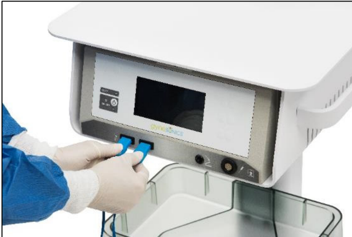
Figure 5-1. Disconnect Dispersive Electrodes Cables from RF Generator.
