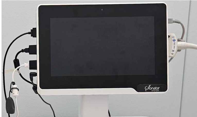
Figure 2-5. Connection ports on the SMART Tablet.
