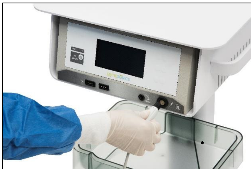
Figure 3-22. Connect RFA Handpiece Cable to front of RF Generator.
