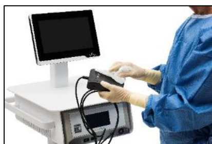
Figure 5-11. Clean parts and external surfaces with a medical grade low alcohol disinfectant.
