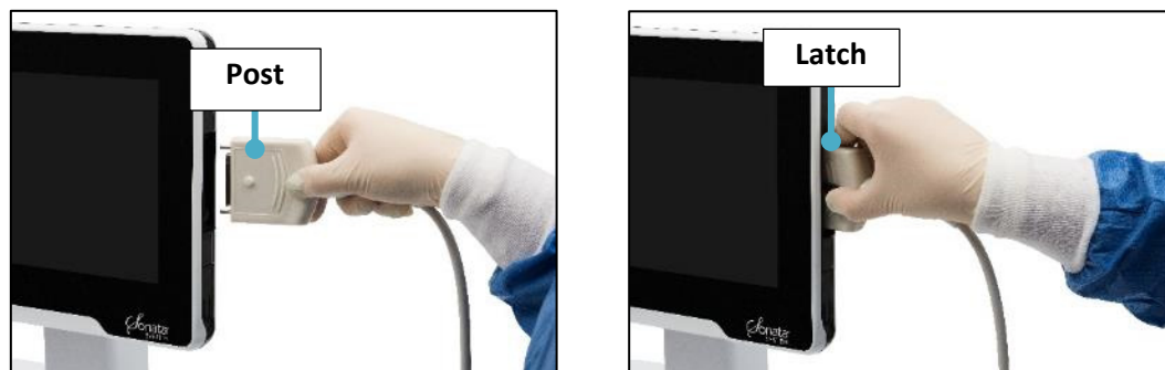
Figure 3-21. Connect IUUS Probe to SMART Tablet and slide latch to lock.
