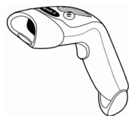
Figure 20: Bar Code Scanner
