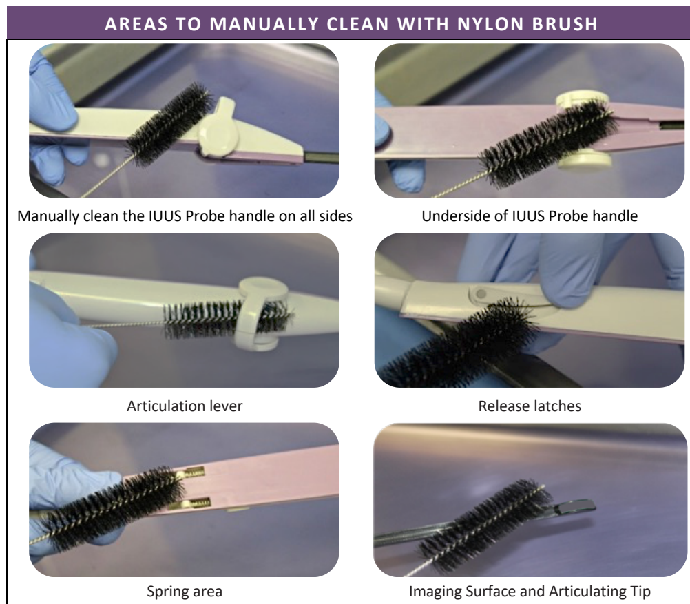
Figure 4-3 Areas of IUUS Probe to manually clean.
