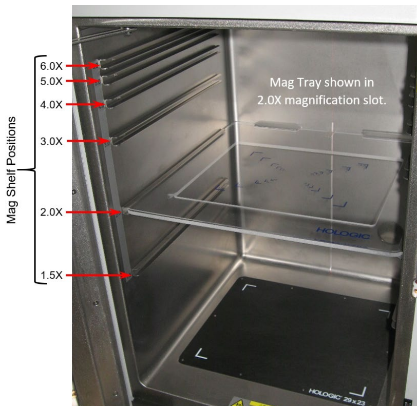
Figure 6: X-Ray Chamber with Magnification Levels
