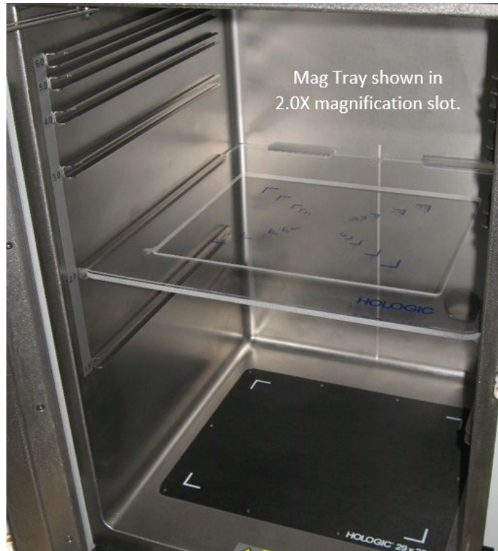
Figure 27: X-Ray Chamber with Mag Tray Installed
