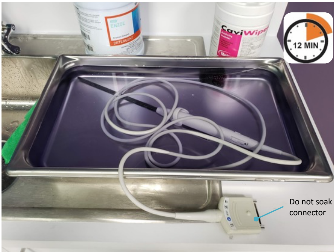
Figure 4-2 Fill with sufficient solution to cover the device.
