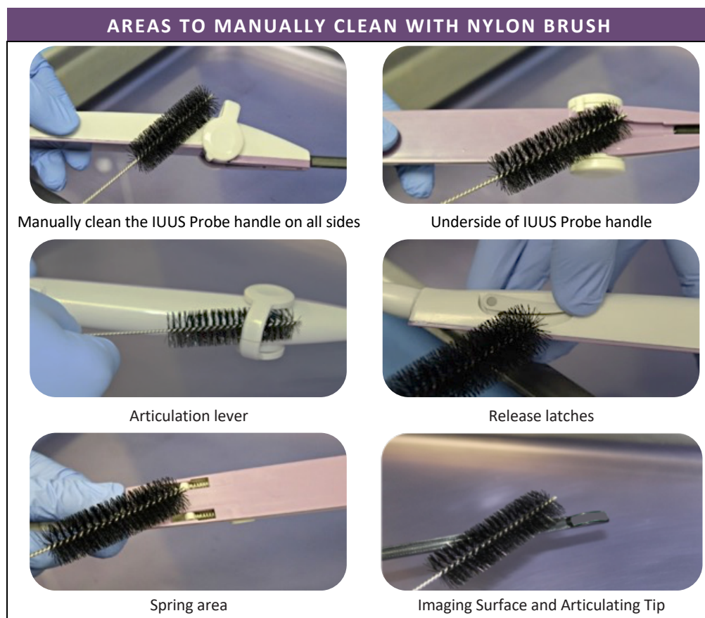
Figure 4-3 Areas of IUUS Probe to manually clean.
