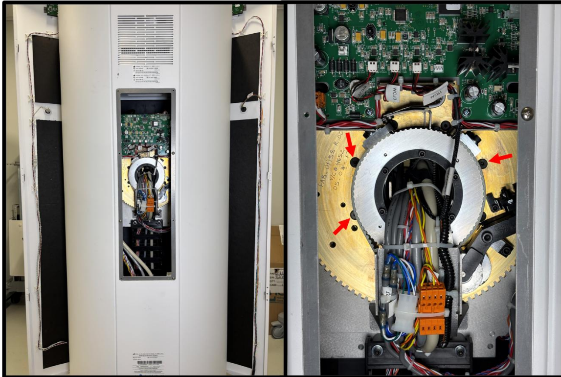
Figure 1 – Back of 3Dimensions with raised C-arm for VTA Access. Red arrows indicate some of the VTA rotation screws
