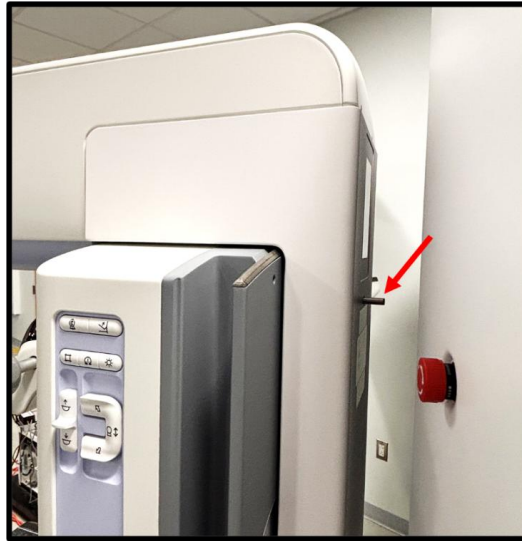
Figure 11 - C-Arm and Tube head positioned at 180° with C-Arm positioned to engage alignment pin
