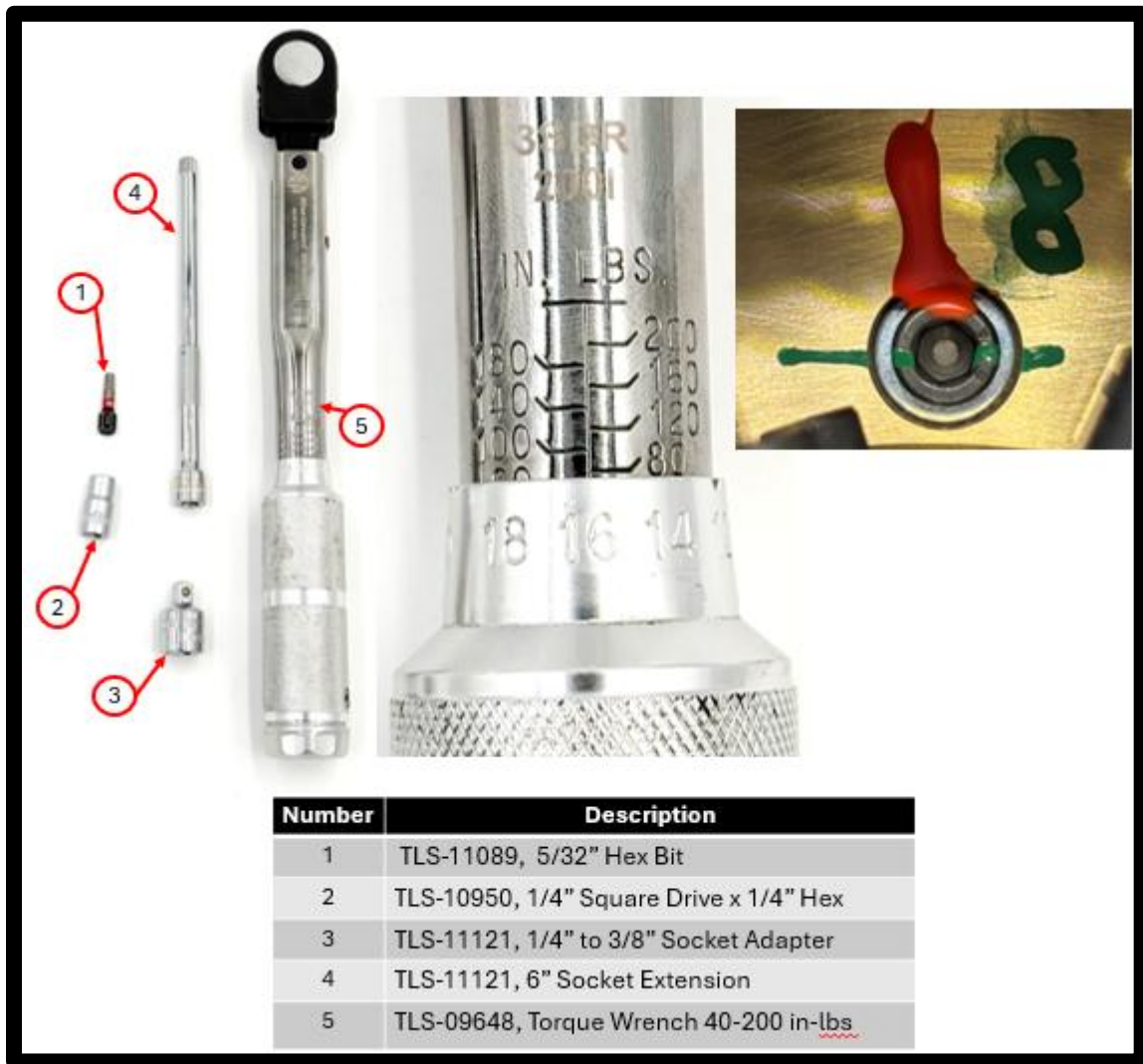
Figure 6 - Socket head hardware torque inspection tools
