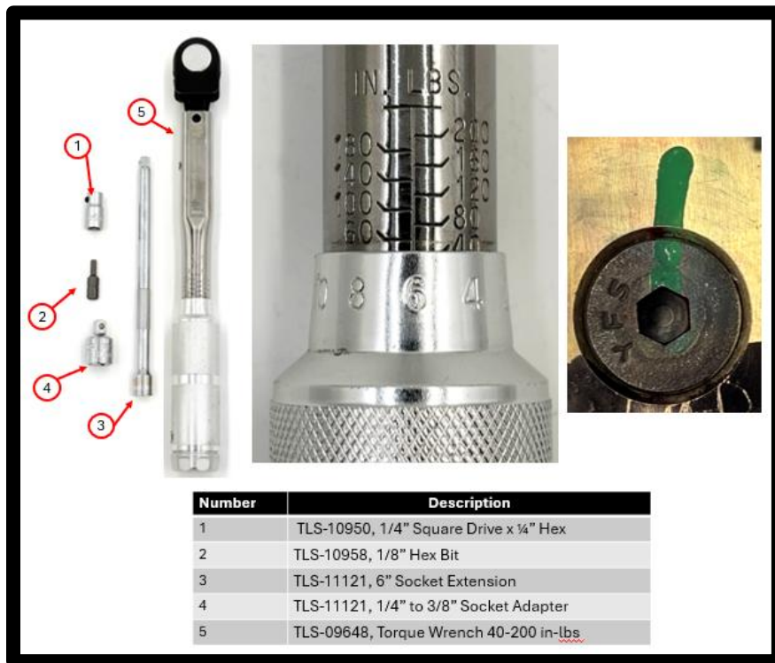
Figure 5 – Flat head hardware torque inspection tools
