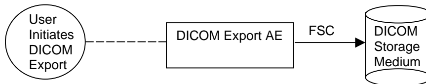
Figure 4.1-1 Application Data Flow Diagram for Media Storage
