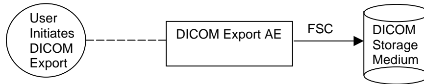
Figure 4.1-1 Application Data Flow Diagram for Media Storage
