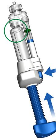
Figure 9: Removing Air from Inflation Device
