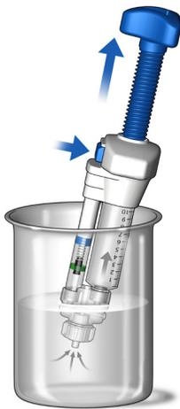
Figure 8: Filling Inflation Device with Saline
