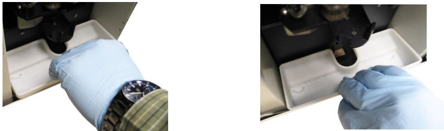
Figure 7-13 Place the Catch Tray into the Cabinet. Fit Screws into the Tray Indents.
