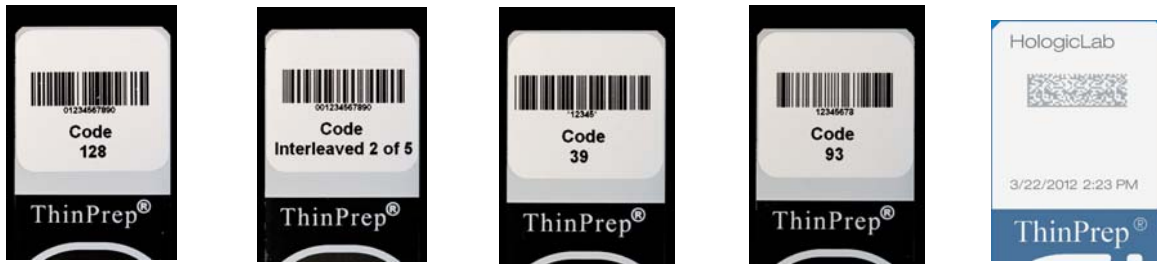
Figure 7-3 Examples of How Barcodes Fit onto a ThinPrep Slide
