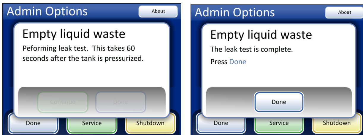
Figure 8-11 Waste System Leak Test
