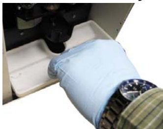
Figure 7-13 Place the Catch Tray into the Cabinet. Fit Screws into the Tray Indents.
