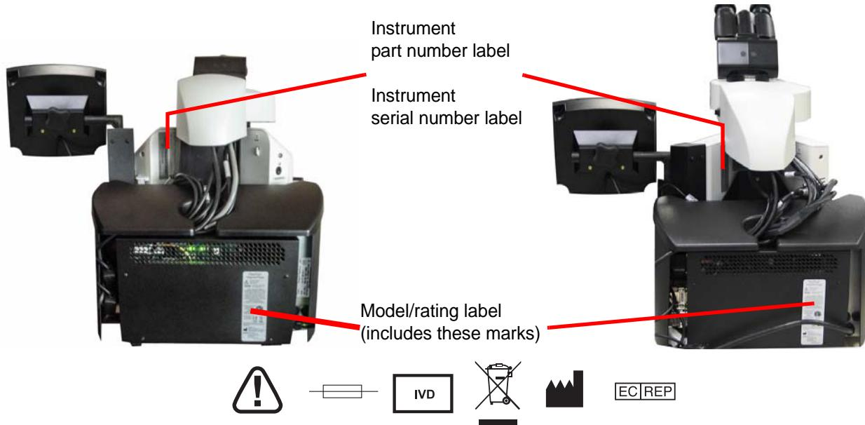
Rear of Instrument (PC removed for clarity.)
