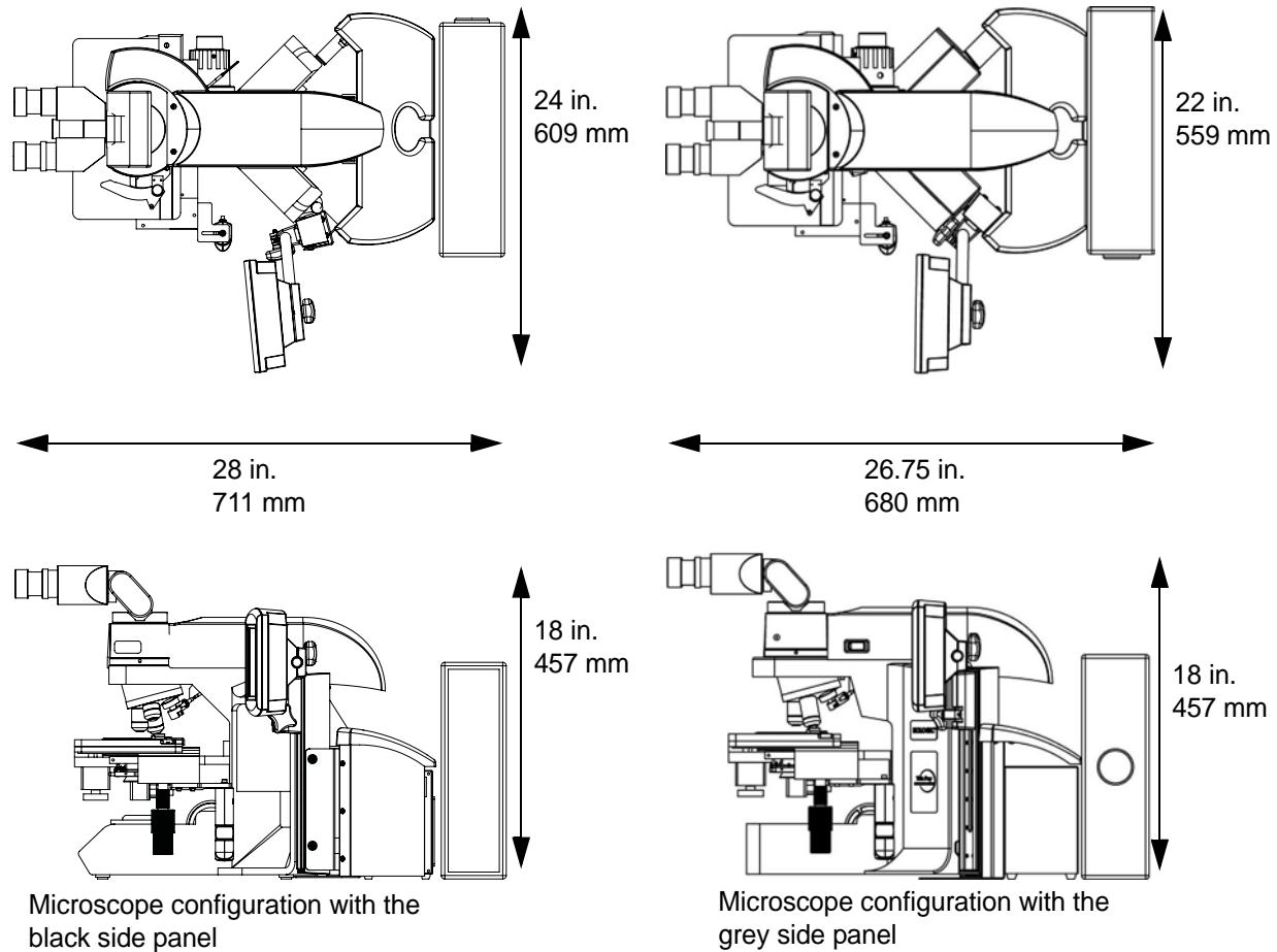
**Figure 1-4 Review Scope Manual+ Dimensions (two microscope configurations shown)**
