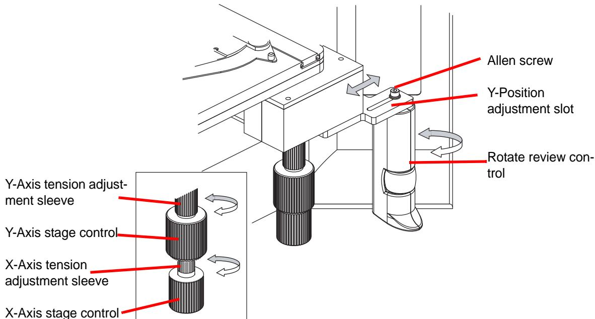
**Figure 2-5 Adjust Substage Controls**
