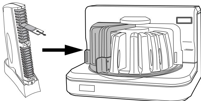
A prepared ThinPrep slide is loaded into a slide cassette, which is loaded into the Image Processing Station.
