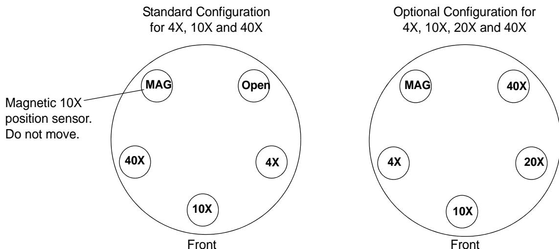
**Figure 2-4 Positions of Objectives in the Nosepiece**
